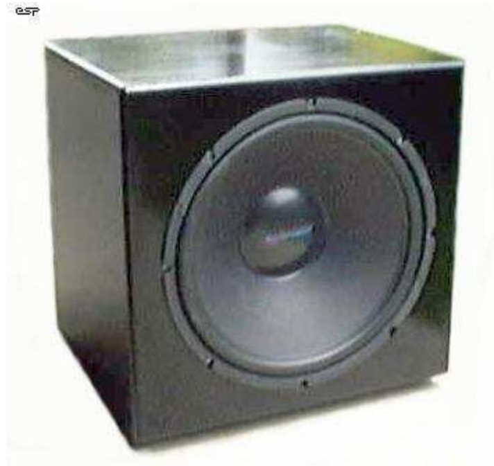
Figure 3 - Photo of Completed EAS Cabinet
